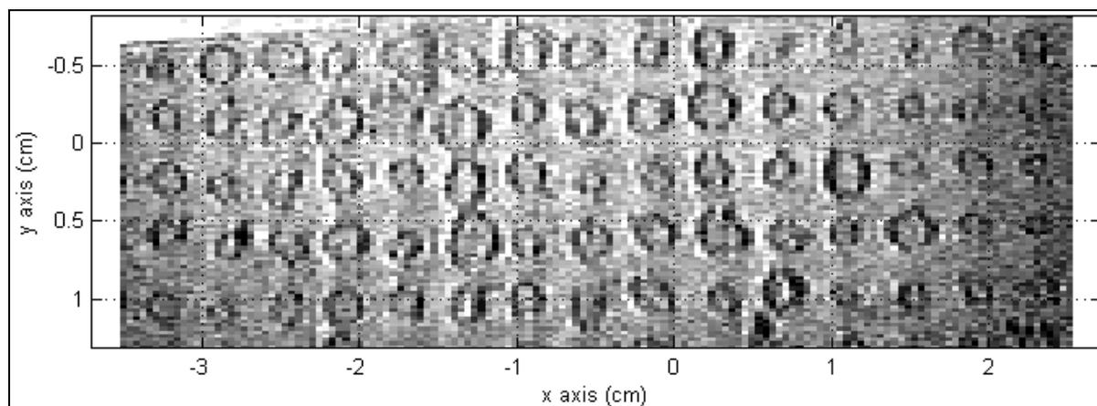
The slide was made by laser etching a 5 x 15 array and spotting with cDNA (all the same). cDNA was then spotted onto the spots directly and allowed to dry. This was subsequently washed before imaging in water. MRI details: RARE sequence, RARE factor = number of lines = 64,  $T_E = 30$  ms,  $T_E^{\text{eff}} = 975$  ms, 8 averages, spatial resolution =  $1172 \times 547 \mu\text{m}^2$ , slice thickness = 0.5 mm, imaging time = 15.5 s.
