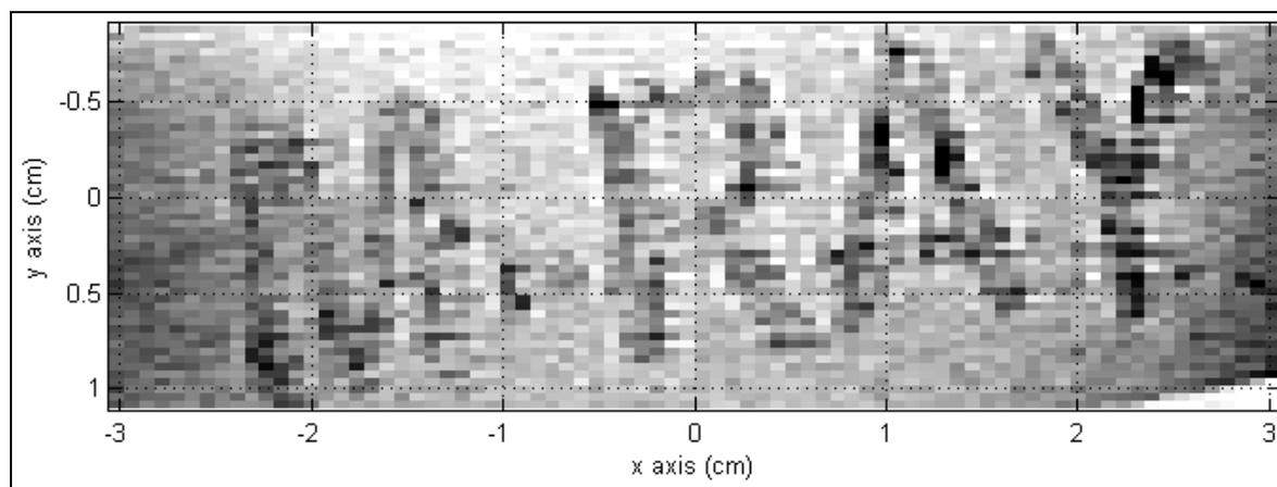
The slide was made by laser etching “M-RAY” the glass slide, and then immobilising cDNA into the etch surface before hybridising with cDNA (as described in the communication) and imaging in water. MRI details: RARE sequence, RARE factor = number of lines = 128,  $T_E = 30$  ms,  $T_E^{\text{eff}} = 1726$  ms, 16 averages, spatial resolution =  $781 \times 391 \mu\text{m}^2$ , slice thickness = 1 mm, imaging time = 62 s.
